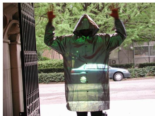
Fig.16 Optical camouflage using RTP..
