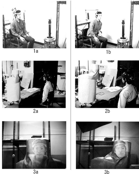
Fig. 13 Experimental Results: (1a, 1b) Human User A at Local Cockpit(A), (2a, 2b) Human User B and Telexistence Robot A' in Environment[B], and (3a, 3b) the image of the human user A on the robot A'. A black dot is where the camera is located.
