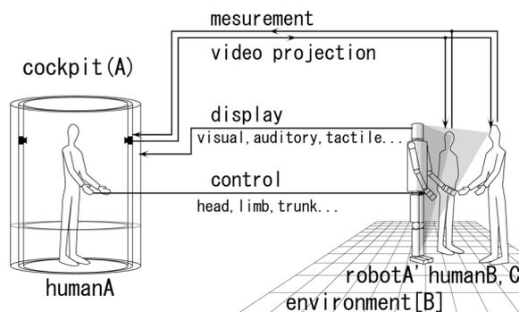
**Fig.24 Schematic diagram of TWISTER used as a cockpit for robotic mutual teleexistence.**
