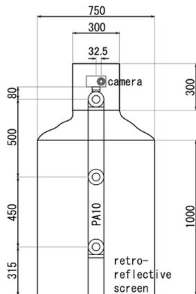
Fig.12 Configuration of Retro-reflective Screen Robot.
