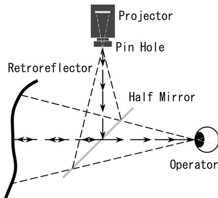
Fig.14 The principle of RPT system.
