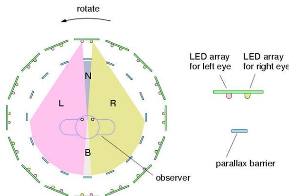
**Fig.20 Principle of autostereopsis using moving parallax barrier.**
