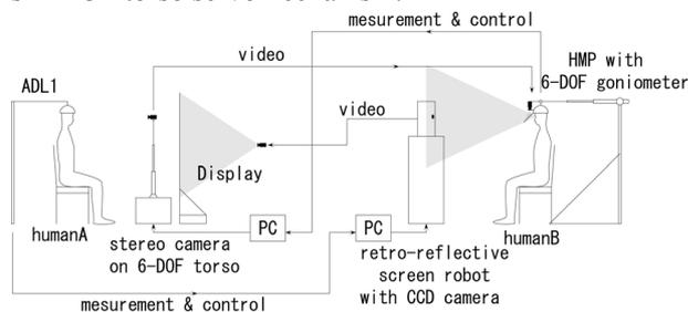
**Fig. 9 Schematic Diagram of the Robotic Mutual Telexistence system Experimentally Constructed [27].**
