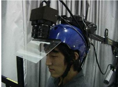
Fig. 11 General View of Head-Mounted Projector (HMP) used in this configuration.
